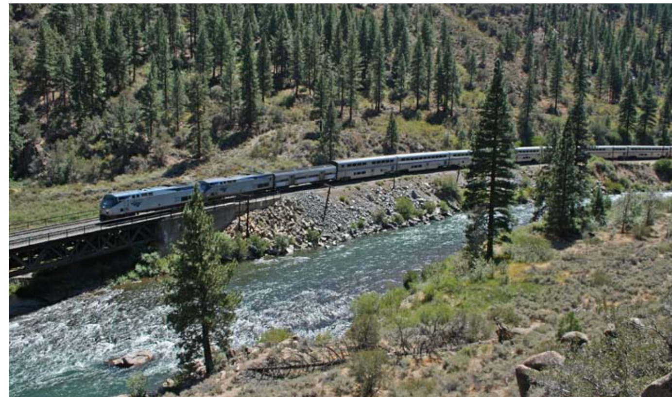
In the mountains, track often follows a river or creek as it does here, at the east end of Donner Pass. Following the flow of water often shows the easiest way over a hill and the gentlest grade.
